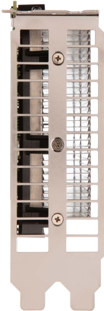
Figure 3. Tesla K20 Bracket
